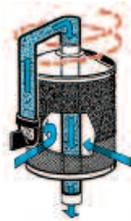
The silver sieve in the PROFI-PLUS is cleaned using a point-rotation-system. Three small jets blast clean filtered water back through the sieve while flushing the residue out through the other side directly into a drain. This is the most advanced system available and is unique to JUDO's PROFI-PLUS.
